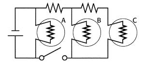
7. Which bulb or bulbs will have a current in the schematic diagram shown above?
