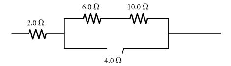
16. What is the equivalent resistance for the resistors in the figure shown above?
