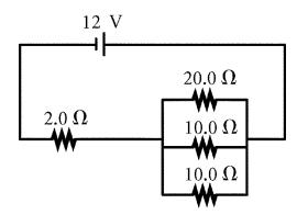
17. How much current is in one of the  $10 \Omega$  resistors in the diagram shown above?
