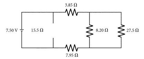
21. What is the current through the 8.20  $\Omega$  resistor in the circuit shown above?
